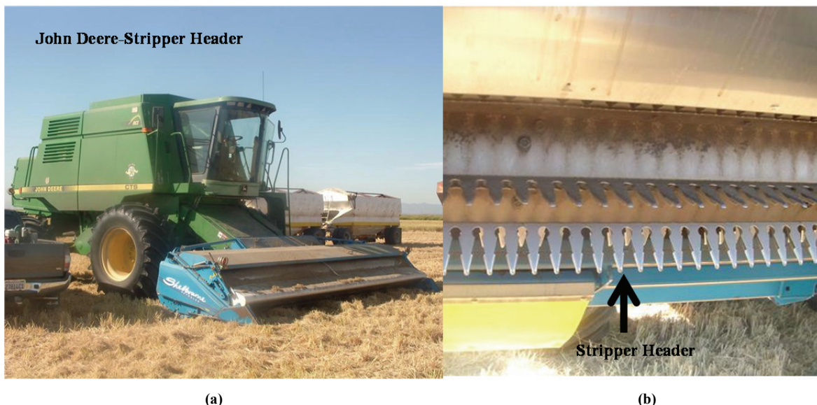
Figure 2. Rice harvester of John Deere (2011) model mounted with a stripper header (a) and magnification of the stripping knife section (b).
