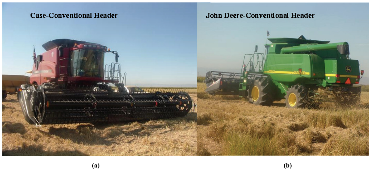
Figure 1. Rice harvesters of (a) Case (1999) and (b) John Deere (2007) models mounted with conventional headers.
