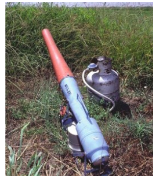
Figure 2. Air cannon used for frightening waterfowl.
