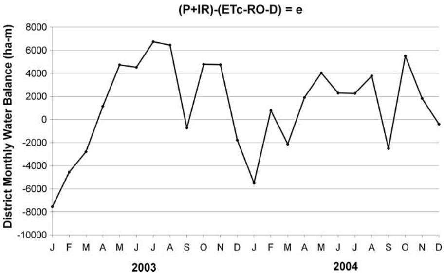
**Figure 12** Error factor: Total monthly district flows. Note: P = precipitation; IR = irrigation; ETc = crop evapotranspiration; RO = runoff; D = percolation; e = error.
