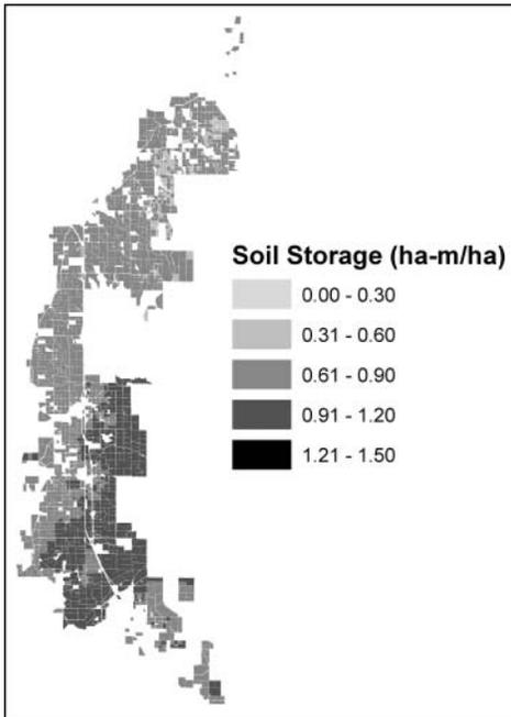
**Figure 10** Glenn-Colusa Irrigation District (GCID) saturated soil storage. Sources: GCID (2004b, 2005); Soil Survey Staff, Natural Resources Conservation Service, and United States Department of Agriculture (2007a, 2007b).
