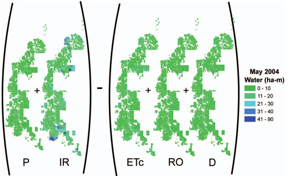
**Figure 11** Adding May 2004 water-balance layers (ha-m). Note: P = precipitation; IR = irrigation; ETc = crop evapotranspiration; RO = runoff; D = percolation. Sources: Glenn-Colusa Irrigation District (2004b, 2005); Soil Survey Staff, Natural Resources Conservation Service, and United States Department of Agriculture (2007a, 2007b); University of California Integrated Pest Management (2006).
