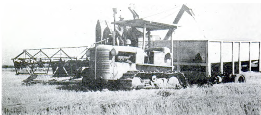
Figure 13.—Transferring rice into a bank-out bed from a combine.
