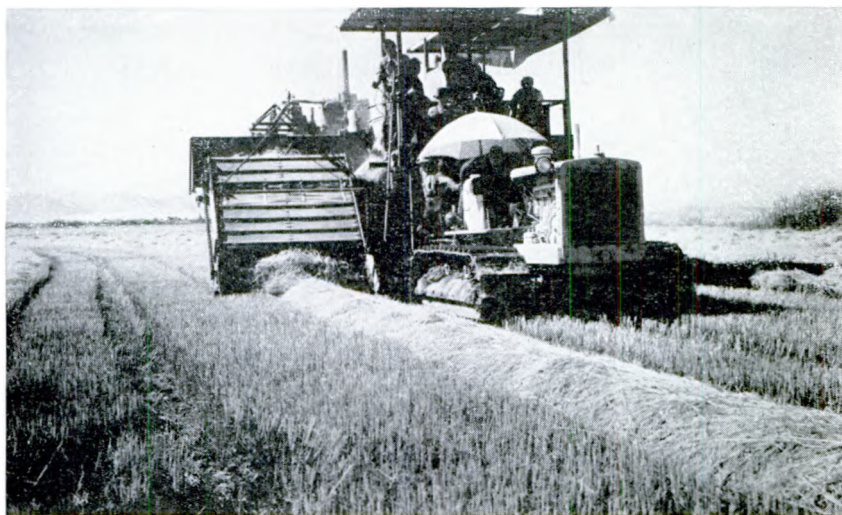
Figure 17.—Threshing rice from the swath in California with a combine with pick-up attachment.
