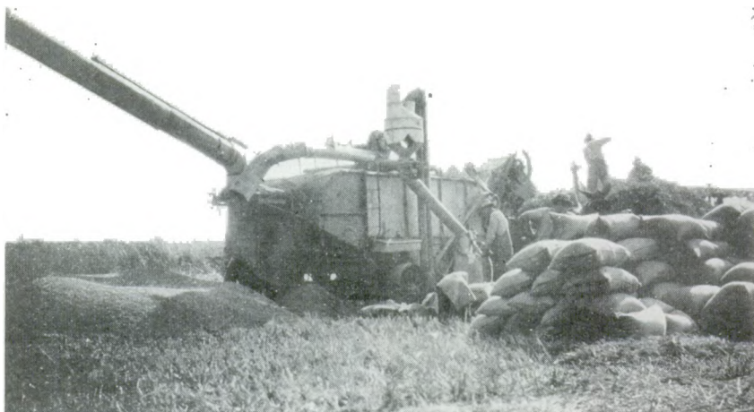
Figure 19. —Threshing rice with a stationary thresher equipped with an aspirator, which is removing material from the grain (left).
