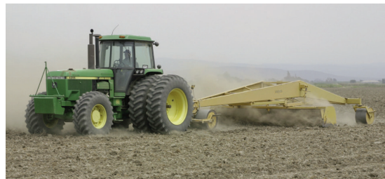
Figure 4. Typical three wheel land plane.
