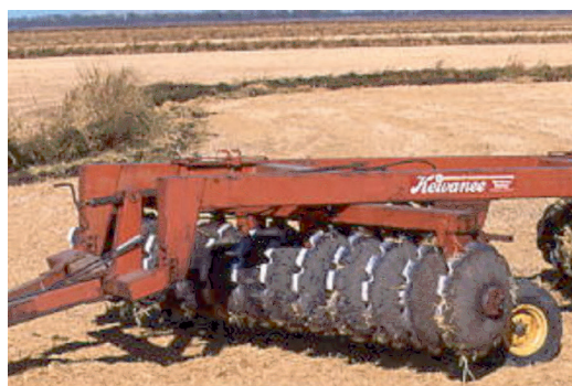
Figure 2. Heavy-duty single offset disc, called a stubble disc, for use in fall straw incorporation (left). Lighter versions with smaller blades are used for spring tillage. On the right, a schematic overview of a typical single offset disc.
