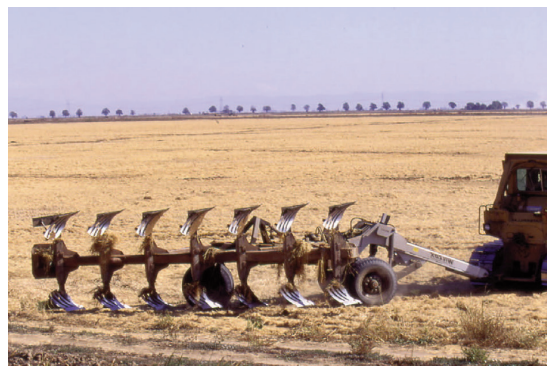
Figure 3. Typical two-way moldboard plow.
