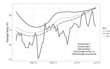
HOBO soil temperature sensors placed 2-inches below the soil surface
