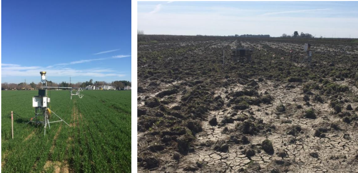
Figure 2. Evapotranspiration measurements using eddy covariance stations in winter wheat and fallow fields
