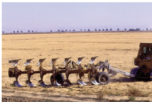
Figure 3. Typical two-way moldboard plow.
