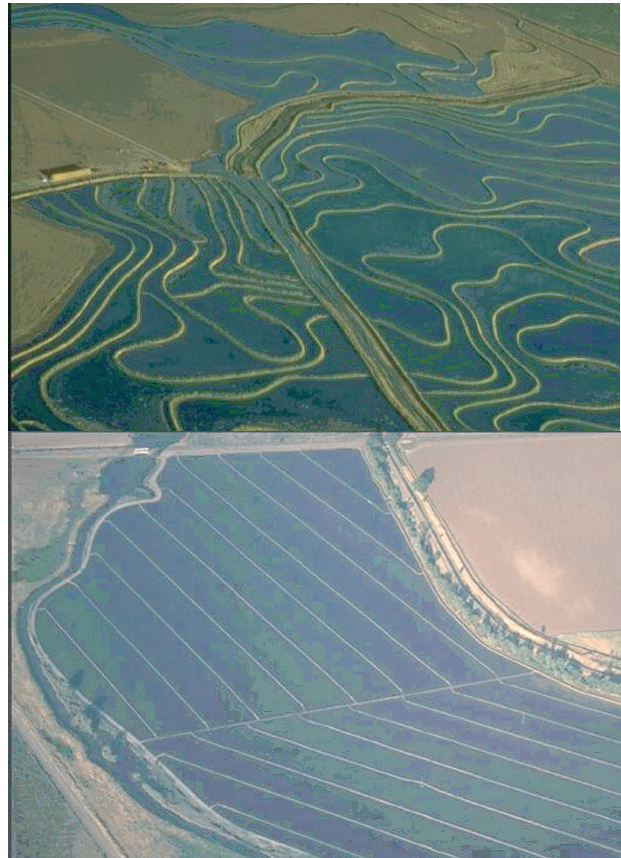
Figure 1. Typical contour levees required in unleveled land, above. Land leveled to uniform slope with parallel levees, below.
