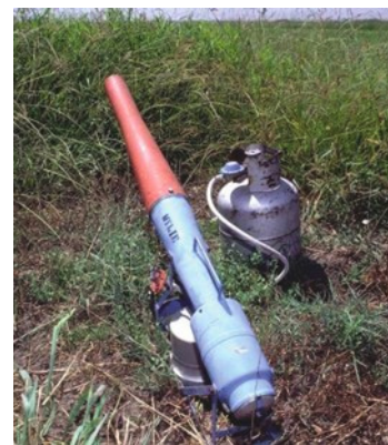
Figure 2. Air cannon used for frightening waterfowl.
