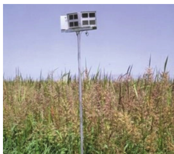
Figure 3. Electronic noise maker.
