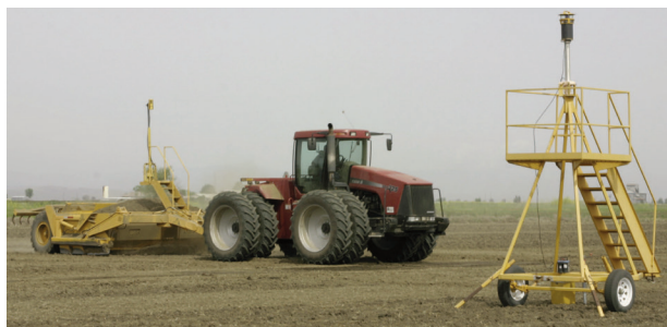
Figure 2. Typical scraper for leveling equipped with laser receiver that guides position of cutting blade. Signal is received from laser beam on stand in foreground. Scrapers may be equipped with single, dual or satellite guided receivers
