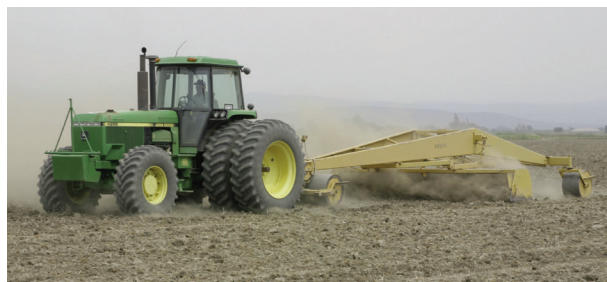
Figure 4. Typical three wheel land plane.
