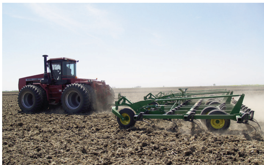
Figure 1. Fall chisel plow operation incorporating rice straw (left), and typical chisel shank (right).
